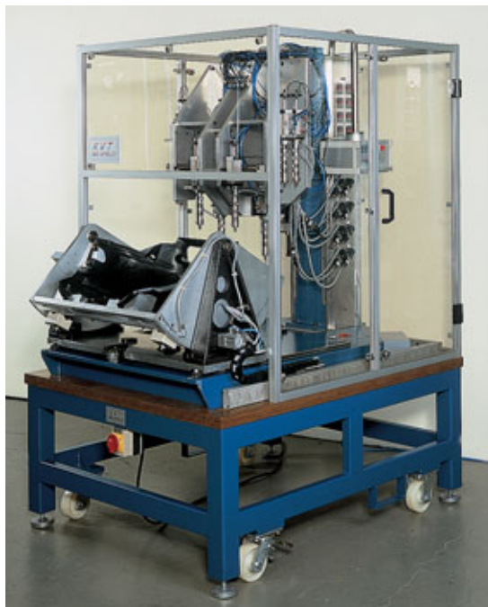
10-item thermal installation (HES) semi-automatic
